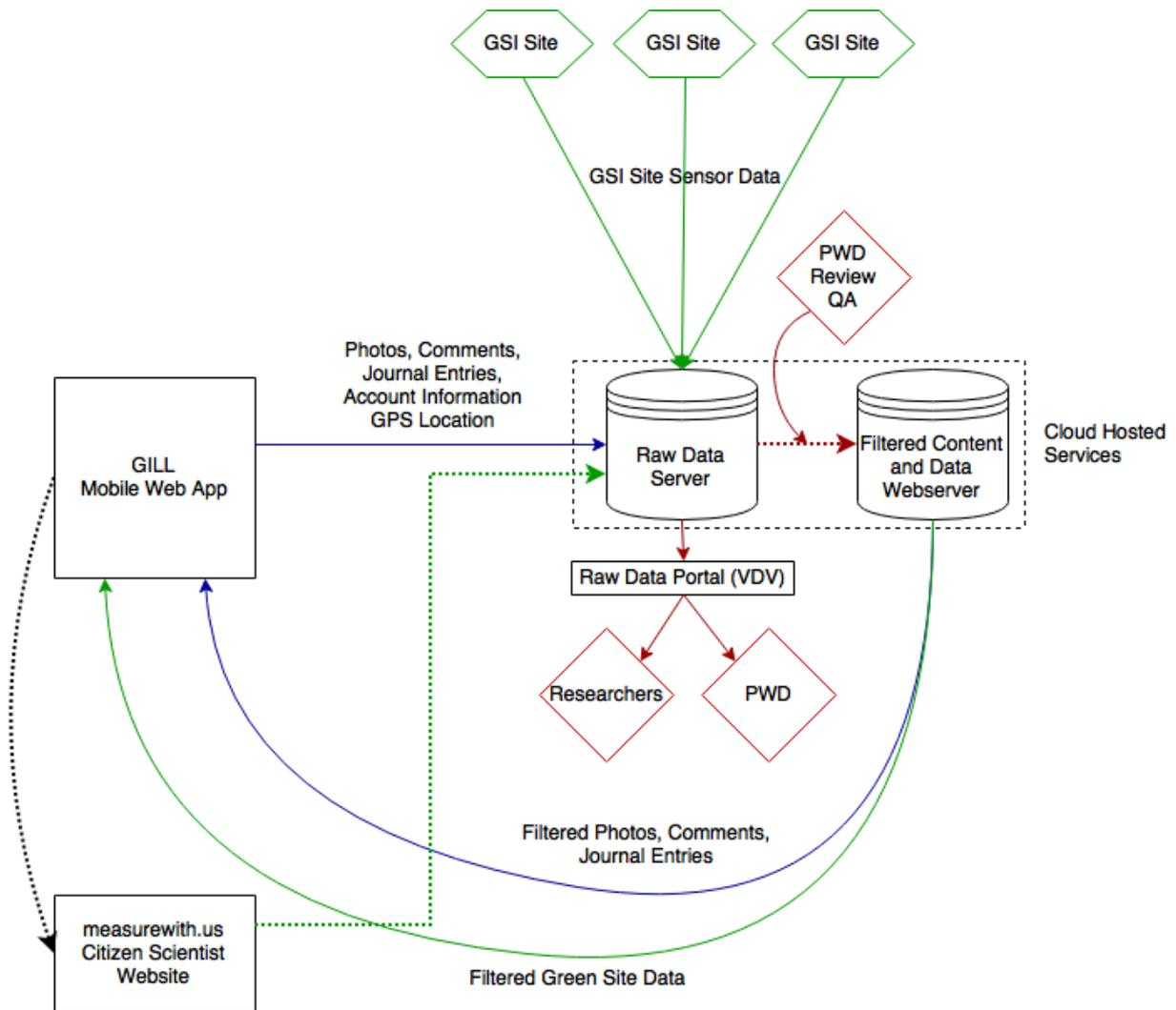
Figure 4- System architecture diagram for web-based services that form the “back end” of the GILL mobile web application.
