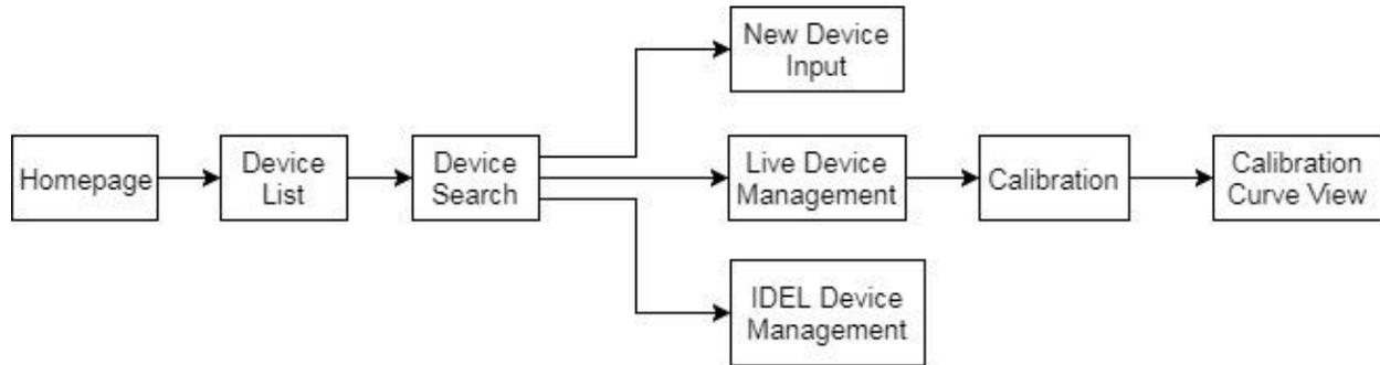
Figure 5- Arrangement of various functions for the device management for admin users
